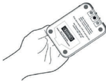
Connect and test the continuity alarm
