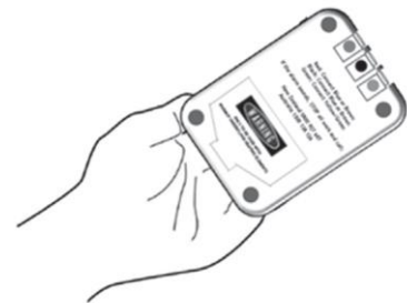
Connect and test the continuity alarm
